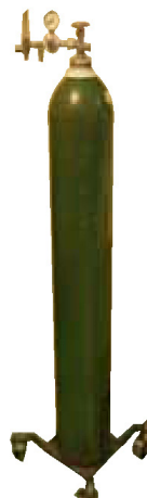
The "H" tank holds 244 cubic feet of oxygen. It weighs about 135lbs.
